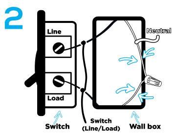
Unscrew and disconnect the wires from the old switch using a screw driver.
