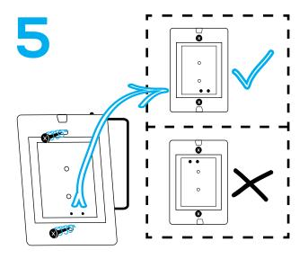
Push all the wires back into the wall box and try to allow as much space for the switch as possible.
