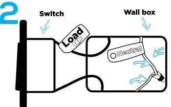
Unscrew and disconnect the wires from the old switch using a screw driver.
