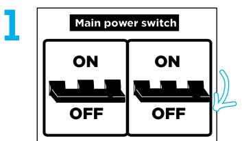
Turn off the power at the circuit breaker for the switch you are replacing.
