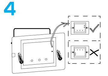
Push all the wires back into the wall box and try to allow as much space for the switch as possible.
