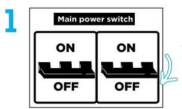
Turn off the power at the circuit breaker for the switch you are replacing.
