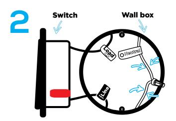
Unscrew and disconnect the wires from the old switch using a screw driver.
