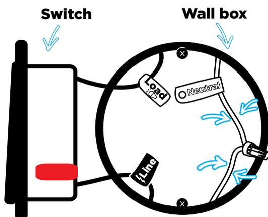
Unscrew and disconnect the wires from the old switch using a screw driver. Remember that you **must** have a Neutral wire to install iotty Light Switch.
