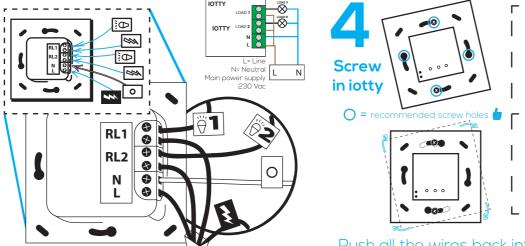
Push all the wires back into the wall box and try to allow as much space for the switch as possible. (Do not push the wires using the back of the switch). Insert the iotty Smart Switch in the wall box screws.
