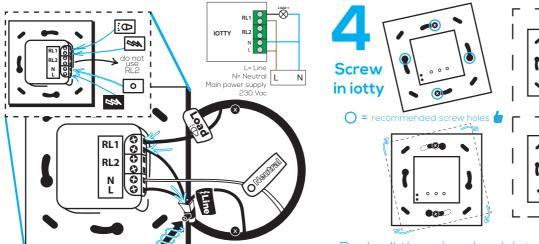
Push all the wires back into the wall box and try to allow as much space for the switch as possible. (Do not push the wires using the back of the switch). Insert the iotty Smart **Switch** in the wall box screws.
