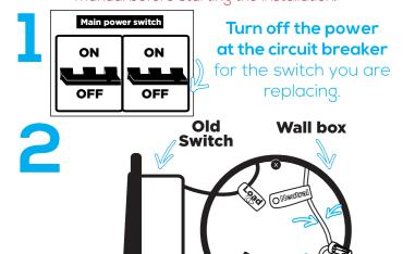
Remove your old switch and label your wires. Remember that you must have a neutral wire to install iotty Smart Switch.
